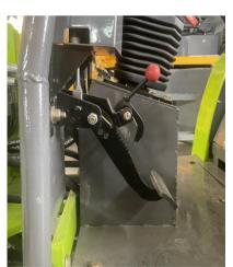
The accelerator pedal is on the right and the brake is on the left hand side of the dash board. The brake also has a manual park brake, controlled by the red handle.
