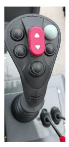
Pull the joystick back to raise the lifting arm and the attachment.
