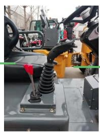
Push the joystick forward to lower the lifting arm and the attachment, pushing to the end is the float position
