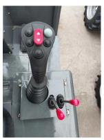
we uses a Quick Hitch system to connect attachments. Attachment must be in an on-ground safe position before using the quick hitch control leaver. Forward movement on the quick hitch handle will release the locking pins to enable removal of the attachment. Always return the quick hitch leaver to its locked position. The hydraulic three way valveleaver needs to be in the Quick hitch position. CAUTION-always ensure the locking pins are correctly in place before using any attachment.
